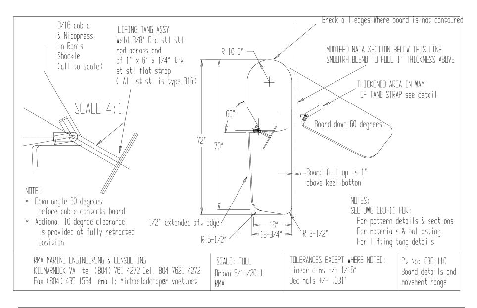
NOTE: I THINK THE ABOVE DWG IS THE BEST DESIGN FOR A BOARD THAT WILL FIT EVERY SEABREEZE WITHOUT ANY SIGNIFICANT COMPROMISES. IF YOU DISAGREE PLEASE L<ET ME HAVE YOUR COMMENTS ASAP. THE DETAIL DRAWINGS SHOWING TANG CONSTRUCTION, PIVOT BUSHING, FOIL SECTION ETC WILL BE COMPLETED FOR THE TWO VENDORS IMMEDIATELY THEREAFTER Michael
